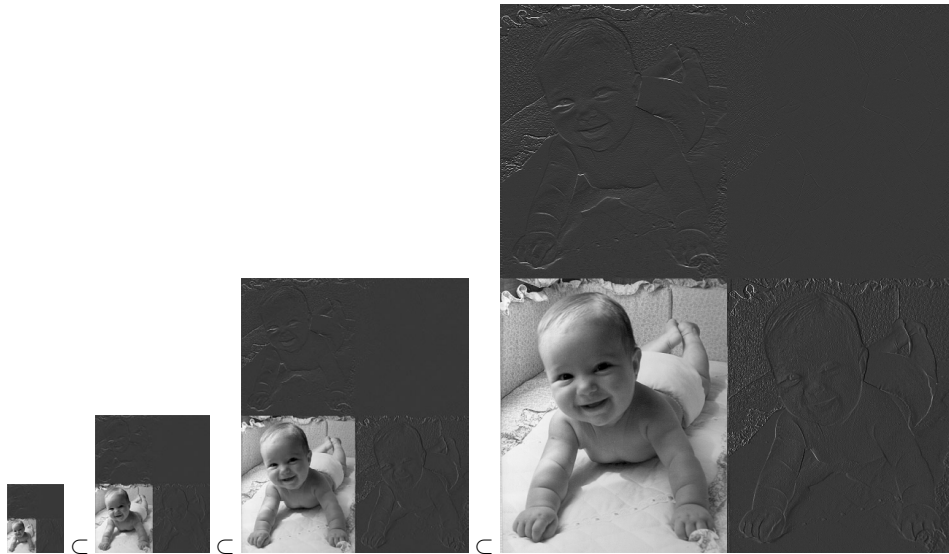
Fig. 13. Nested subspaces in the context of image processing. The details are represented in the grey regions (the contrast was enhanced for better visualization).
