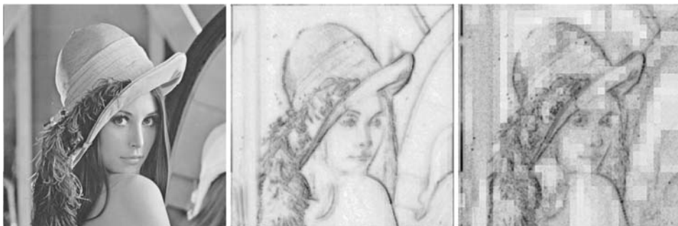
Fig. 8. Original image Lena; mask from Naornita et al., 2006b and Barni's mask for level l=0 . The masks are the complementary of the real ones.
